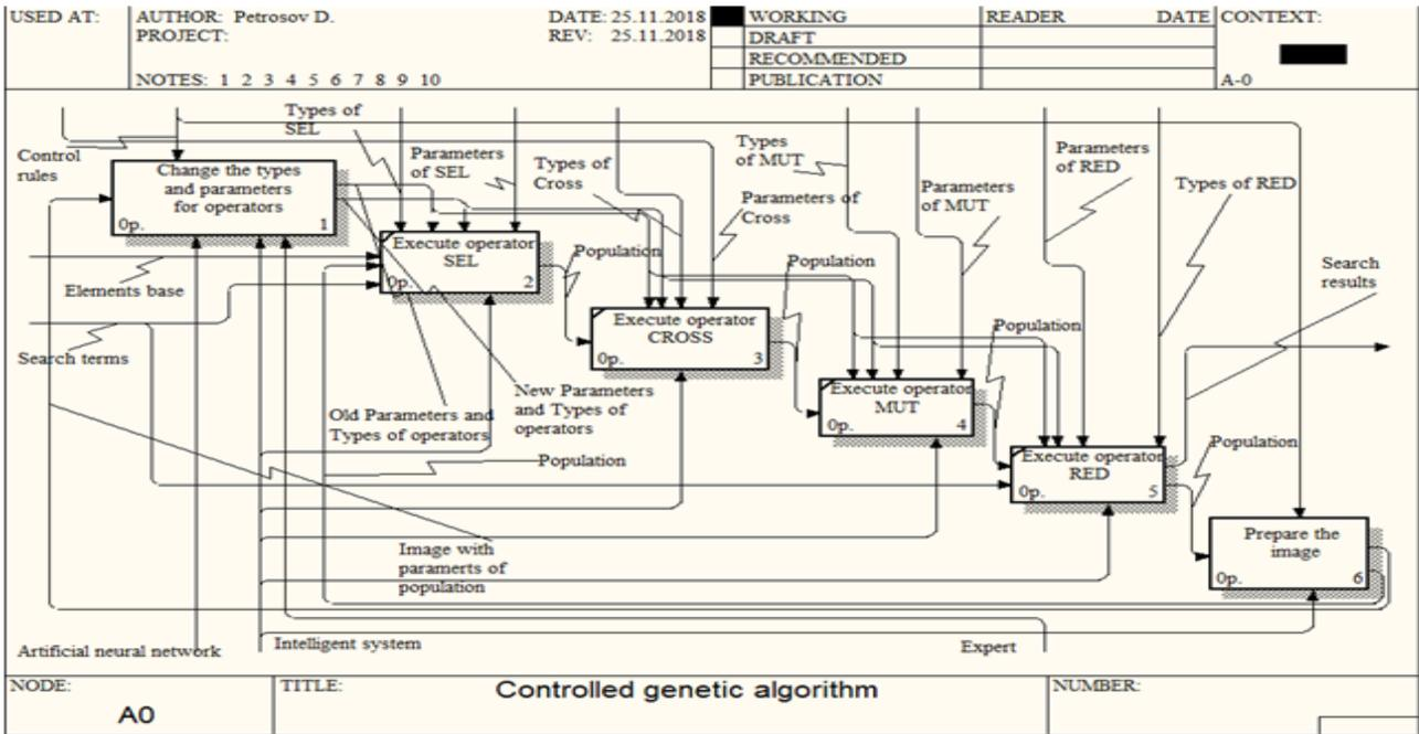
**Figure 2** – The decomposition of the controlled genetic algorithm process
