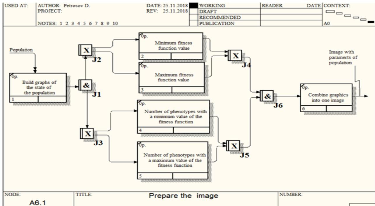
**Figure 3** – The decomposition of the process "Prepare an image"
