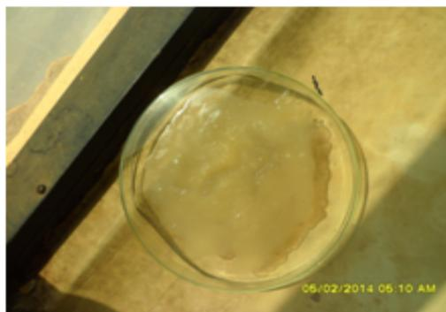
**Fig. 8** PHB Biopolymer layered composites spread and dried in Petri dish
