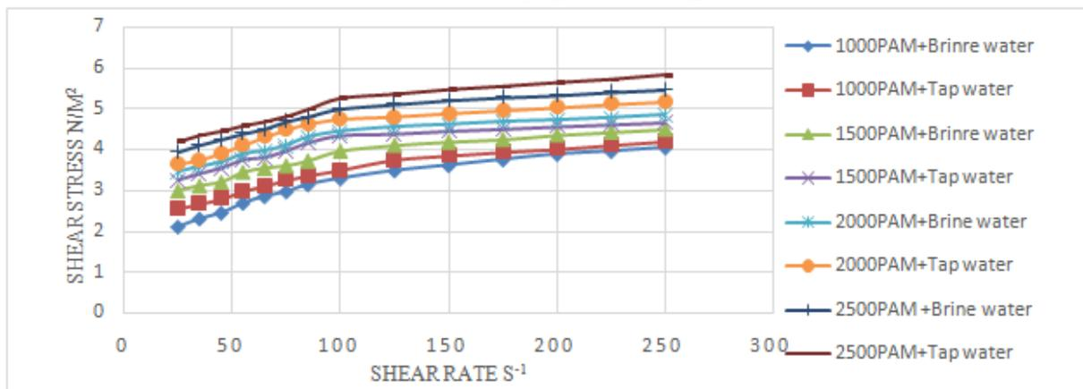
Figure 5:- shear stress against shear rate of different PAM aqueous solutions
