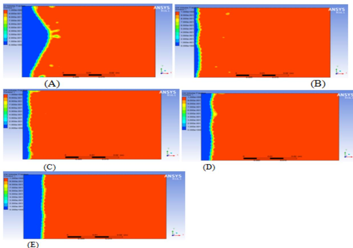
**Figure 7:-** visualization of volume fraction contour for brine water without and with PAM concentrations increases with crude oil, A)brine water, B)1000PAM, C)1500PAM, D)2000 and E)2500 PAM
