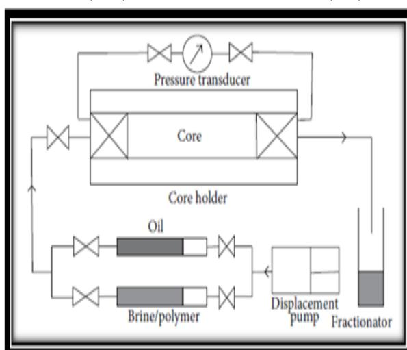
Figure (1): diagram of core flooding schematic[29]
