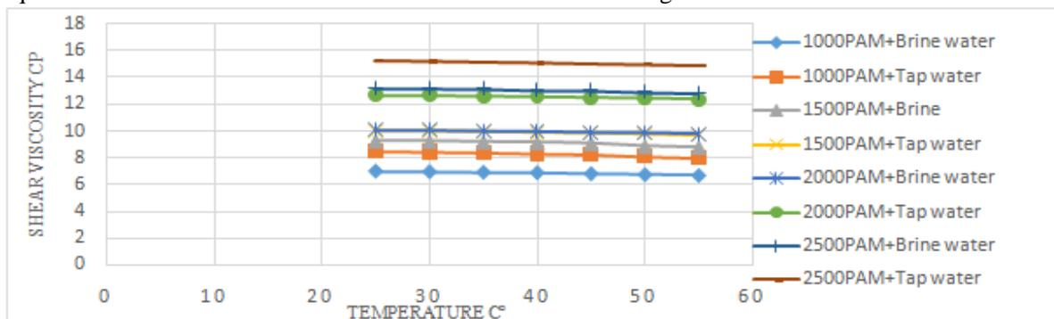
Figure 6:- shear viscosity against temperature of different PAM aqueous solutions at 25 s<sup>-1</sup> shear rate
