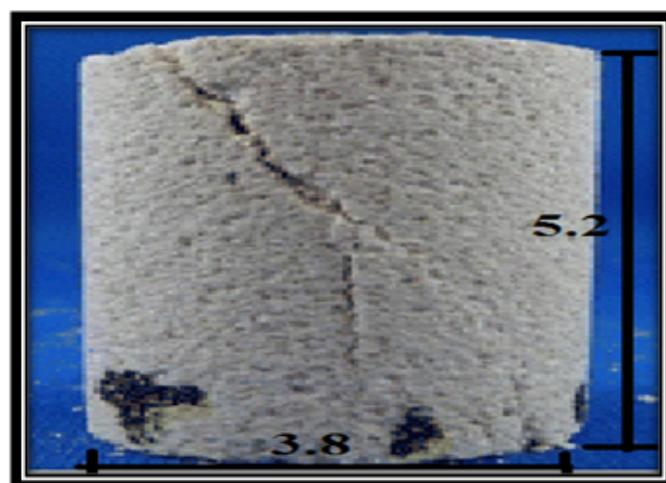
Figure2:- Sandstone core with (5.2) cm length and (3.8) cm diameter
