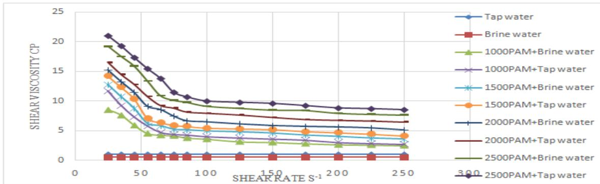
Figure 4:- shear viscosity versus shear rate for different PAM aqueous solutions
