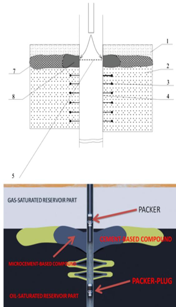
Fig. 4 Torquing the gas isolation shield with the cement slurry. 1 – gas-saturated part; 2 – oil saturated part; 3 – perforations; 4 – production casing string; 5 – GOC; 7 – cementing slurry on the basis of Mikrodur; 8 – cement-based torquing slurry.
