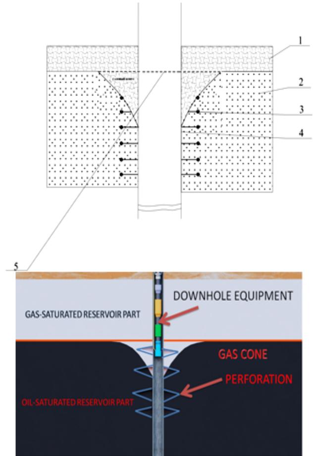
**Fig. 1** The formation of a gas cone in the oil-producing well. 1 – gas-saturated part; 2 – oil saturated part; 3 – perforations; 4 – production casing string; 5 – GOS.
