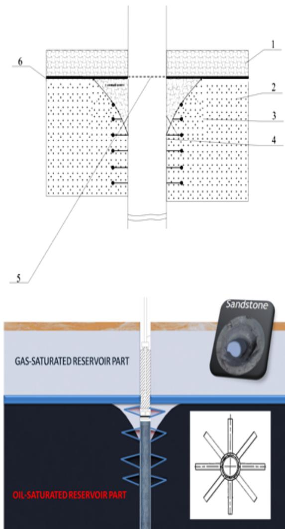
**Fig. 2** Drilling of radial channels at the GOS level. 1 – gas-saturated part; 2 – oil saturated part;
