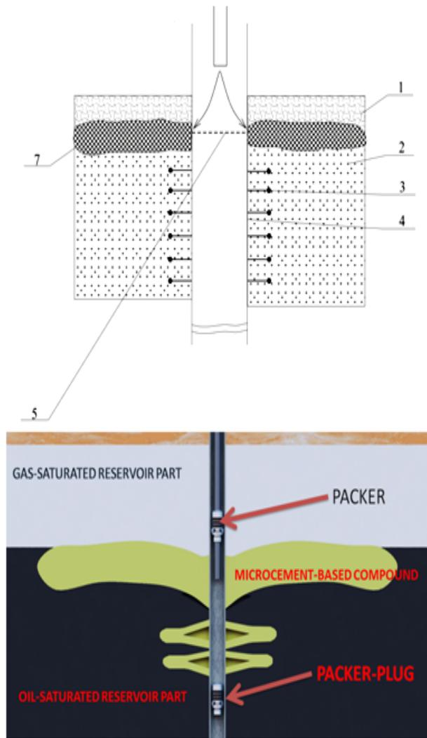
Fig. 3 The injection of the plugging material on the basis of micro-cement. 1 – gas-saturated part; 2 – oil saturated part; 3 – perforations; 4 – production casing string; 5 – GOS; 7 – cementing slurry on the basis of Mikrodur.
