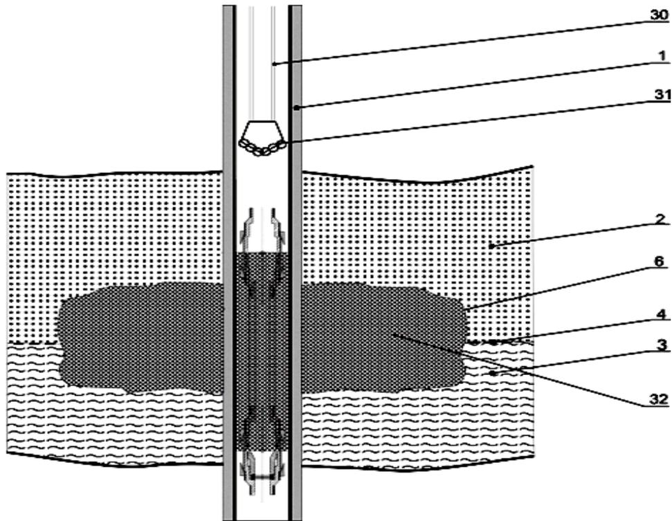
**Fig. 4** Drilling out the packing arrangement with packers. 1 – the well; 2 – the reservoir oil-saturated part; 3 – the reservoir water-saturated part; 4 – OWC; 6 – the perforation; 30 – the drill string; 31 – the milling cutter; 32 – the water-isolating shield.
