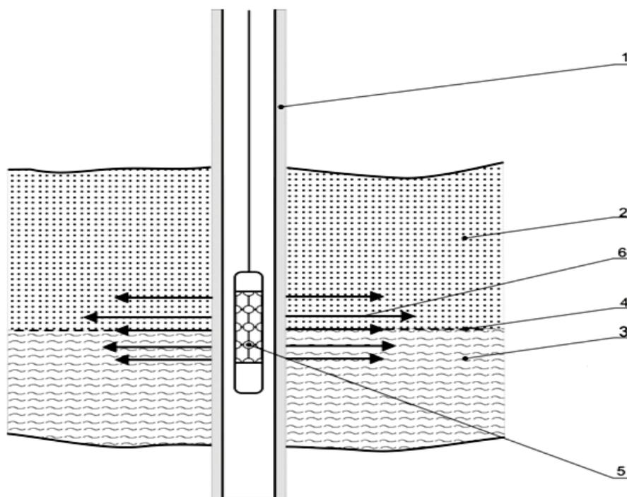
**Fig. 1** Carrying out perforation works in the well at the OWC level. 1 – the well; 2 – the reservoir oil-saturated part; 3 – the reservoir water-saturated part; 4 – OWC; 5 – the perforator; 6 – the perforation.
