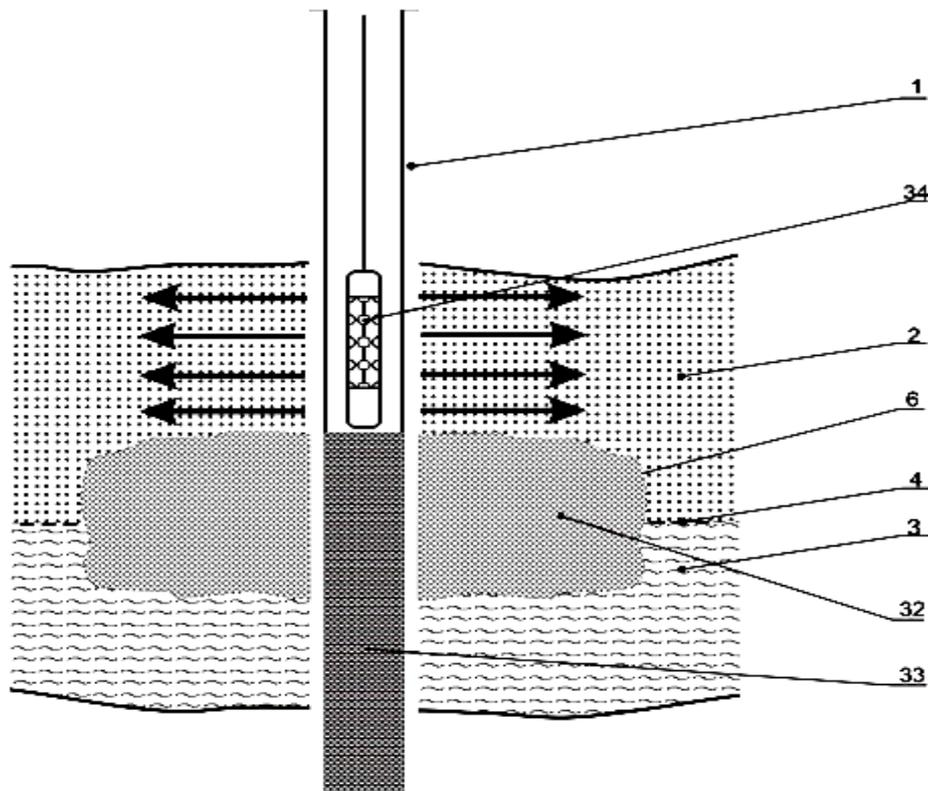
**Fig. 5** Carrying out perforation works in the reservoir oil-saturated part. 1 – the well; 2 – the reservoir oil-saturated part; 3 – the reservoir water-saturated part; 4 – OWC; 6 – the perforation; 32 – the water-isolating shield; 33 – the cement plug; 34 – the perforator.
