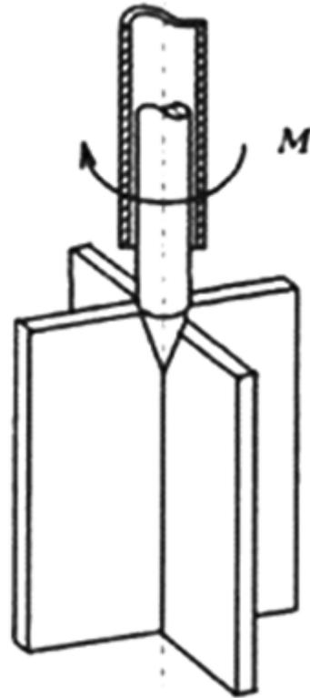
**Fig. 1** Schematic diagram of the impeller device.  $M$  – torque.
