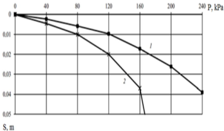
**Fig. 4:** Experimental graphs “settlement-pressure”: 1 is for foundation with contour reinforced sand blanket with the curved floor; 2 is for natural ground.
