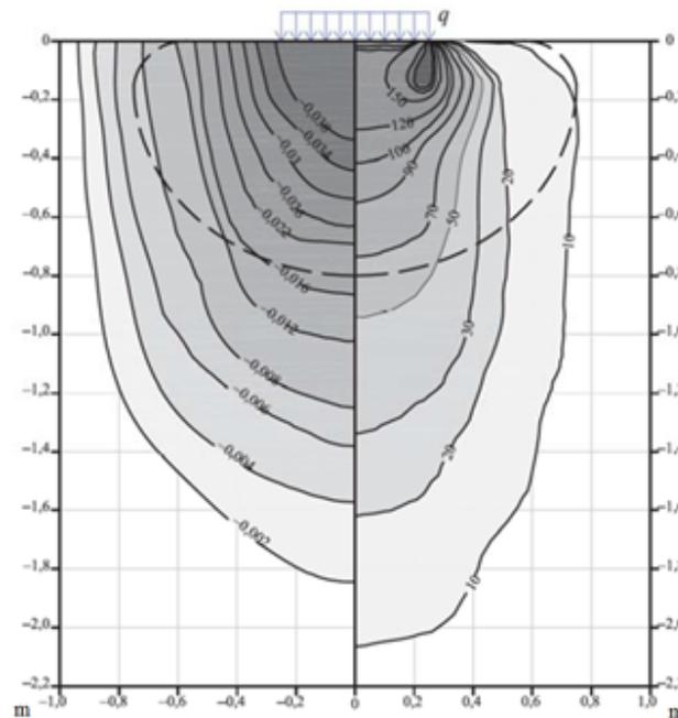
**Fig. 5:** The experimental contour line of the vertical movements (left side, in m) and vertical strains (right side, in kPa).
