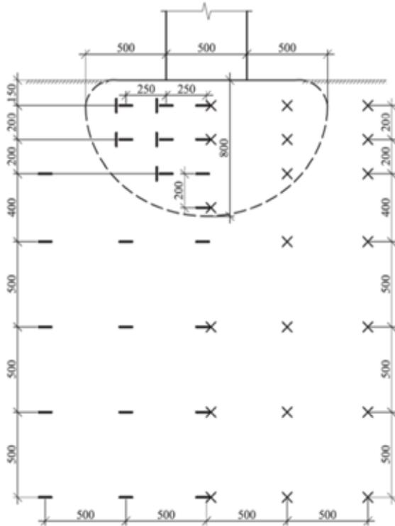
**Fig. 2:** Load cells (on the left side) and ground marks (on the right side) installations scheme.
