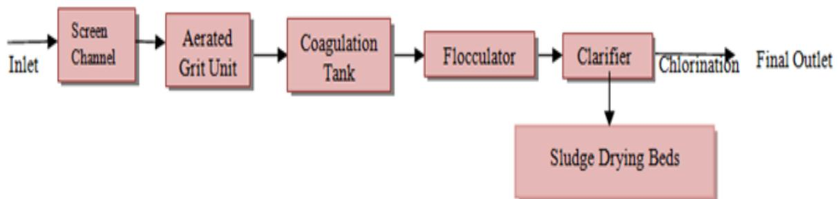
**Fig. 2:** Flow diagram of Liquid Waste Treatment Plant, Hamidia Hospital, Bhopal, M.P., India
