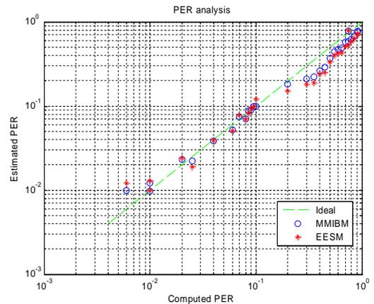
Figure 4. Computed PER vs Estimated PER for 16QAM
