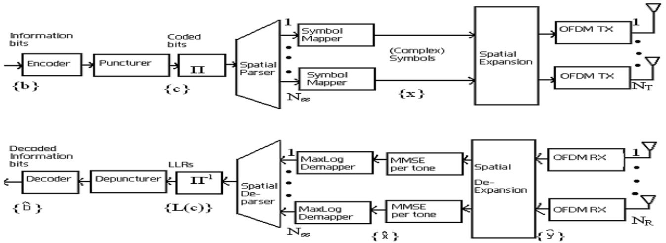
Figure.1 Block diagram of MIMO BICM-OFDM.
