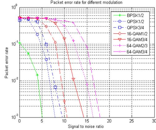
Figure 2. PER vs SNR for various MCS in AWGN channel
