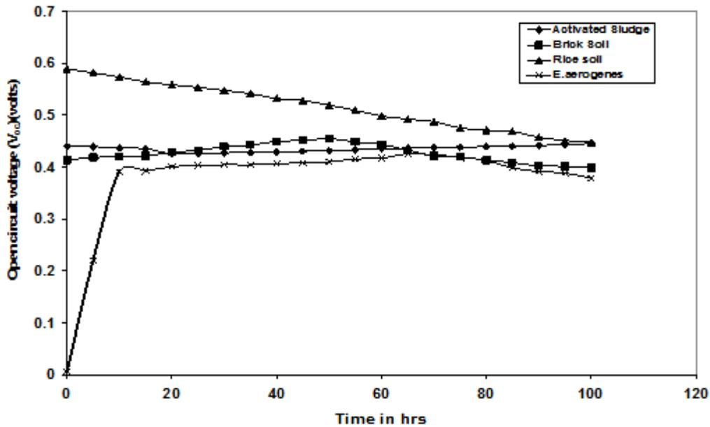
Fig.2 Variation of open circuit voltage with time for dairy waste based MFCs with different cultures from (a) activated sludge from dairy waste disposal plant, (b)brick soil, (c) rice field soil and (d) E. aerogenes.
