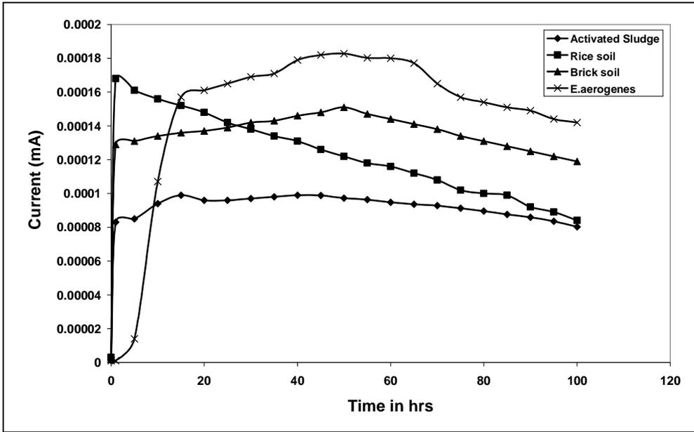
**Figure 3.** Variation of current with time for dairy waste based MFCs with different cultures from (a) activated sludge from dairy waste disposal plant, (b) rice field soil, (c) brick soil and (d) E. aerogenes.
