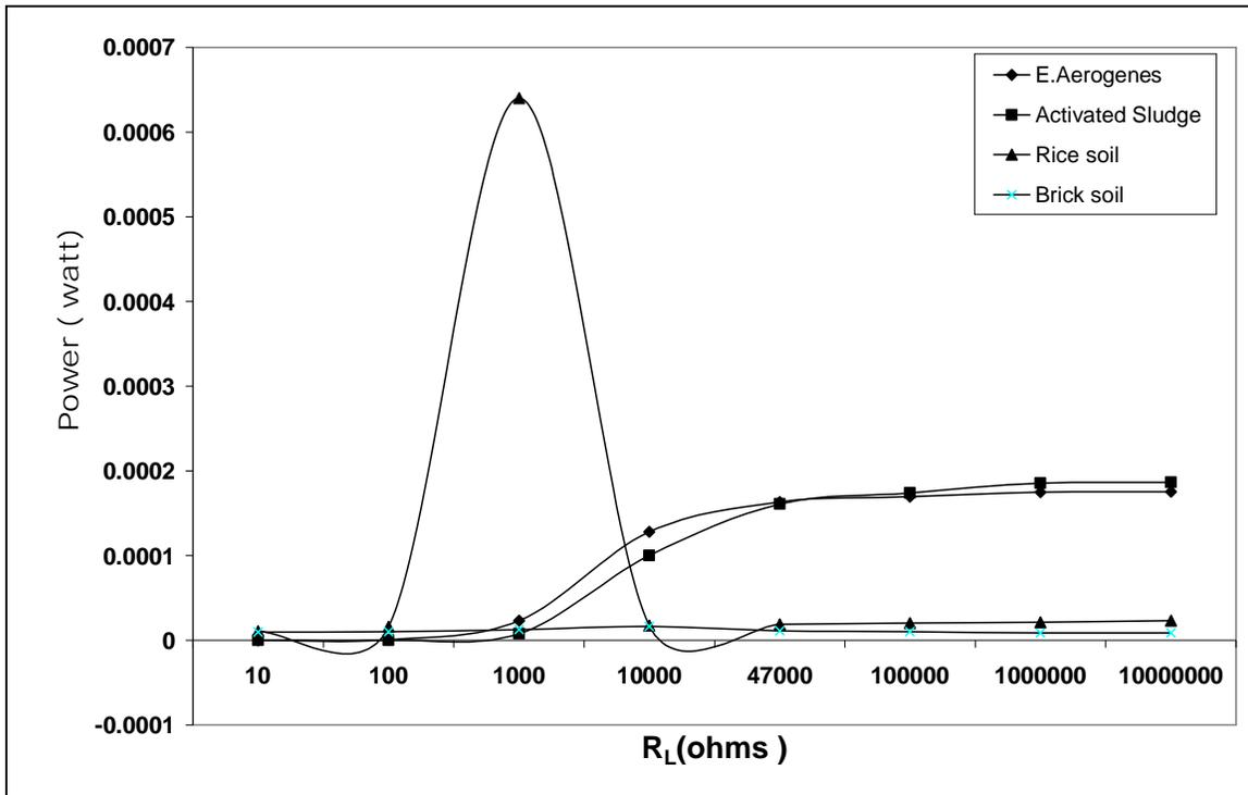
**Figure 5** Variation of power output with load resistance  $R_L$  for the MFCs formed with different cultures (a) E. aerogenes, (b) activated Sludge, (c) rice field soil and (d) brick factory soil.
