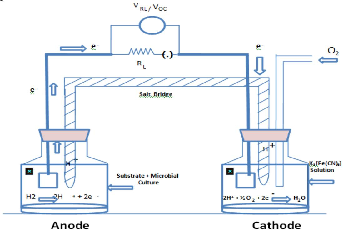
Figure 1 Schematic picture of lab-scale MFC
