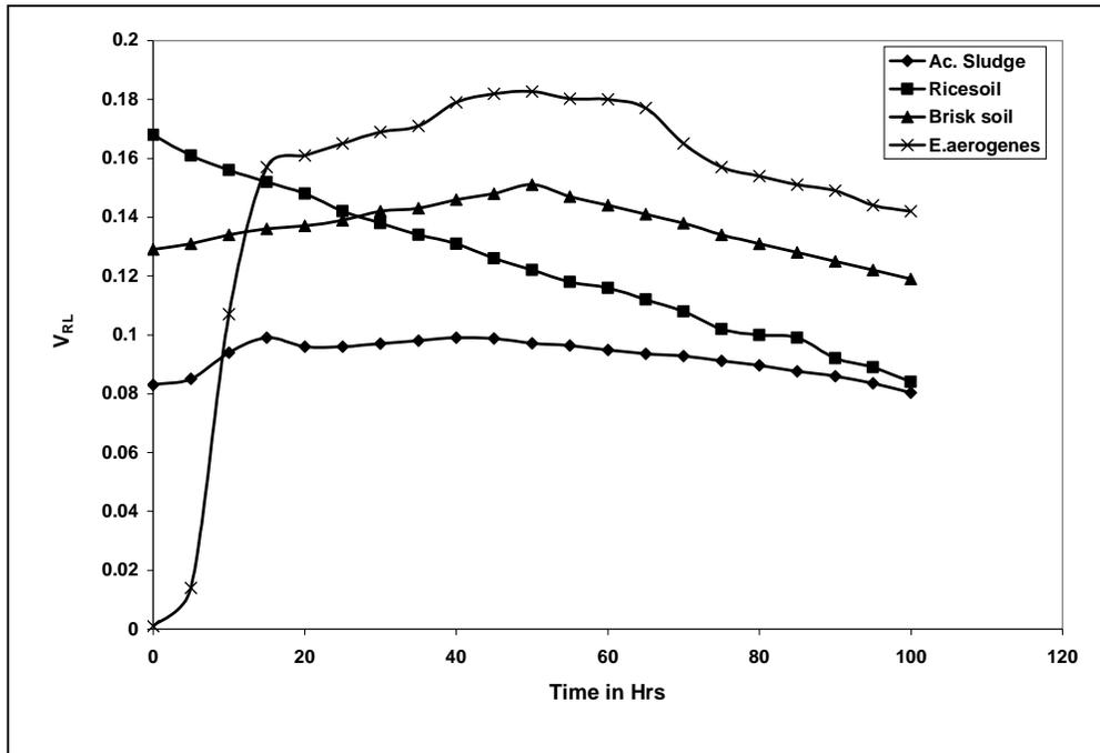
**Fig. 4.** Variation of voltage drop across load resistance  $R_L=1000 \Omega$  with time for dairy waste based MFCs with different cultures from (a) activated sludge from dairy waste disposal plant, (b) rice field soil, (c) brick soil and (d) E. aerogenes.
