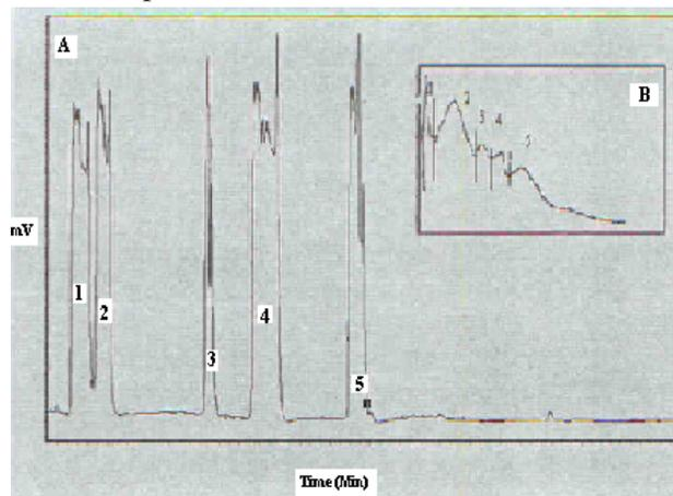
**Fig:4** Electrophoretic pattern of five cephalosporin fractions obtained with the electrophoretic affinity chromatography ( EAC) which was performed on the chemstation software N3000; (a) with pressurized column packing and adsorption on SCX for one hour, ( Insert –B) un pressurized column packing and without adsorption on SCX.
