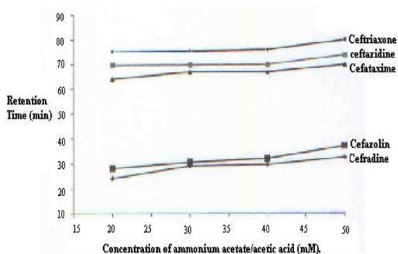
**Fig: 2** Effect of ammonium acetate/ acetic acid concentration in the buffer. Conditions: mobile phase, ammonium acetate/acetic acid (pH 6.0) with 50 % ACN.
