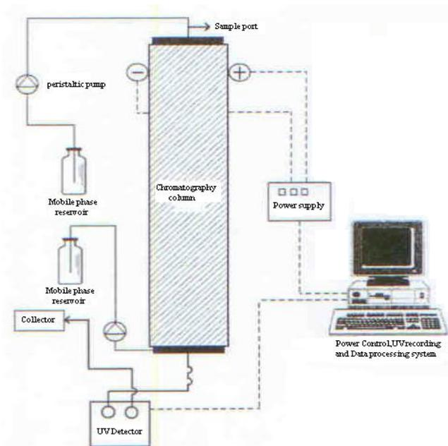
**Fig: 1** Experimental system of electrophoretic affinity chromatography. (Insert) photograph of a specially designed and fabricated glass chromatography column with a length of (250 x 50mm I.D) has been used.
