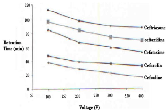
**Fig: 3** Effect of voltage. Conditions: mobile phase, 20mM ammonium acetate/acetic acid, pH 6.0 with 50 % ACN.
