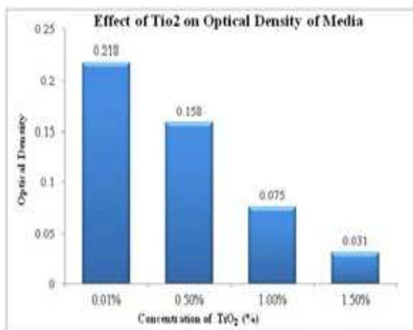
**Fig. 1:** E. coli Density in different TiO<sub>2</sub> concentrations.
