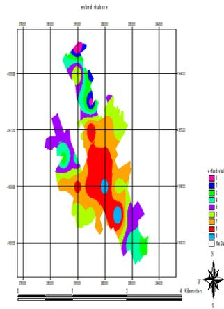
Figure 14: The equivalent sound level (Leq) at night, March the measurement stations based on DBA
