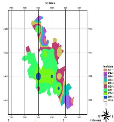
Figure 4: The equivalent sound level (Leq) in the evening of July in measurement stations based on DBA
