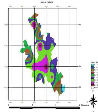
Figure 6: The equivalent sound level (Leq) at night, August the measurement stations based on DBA
