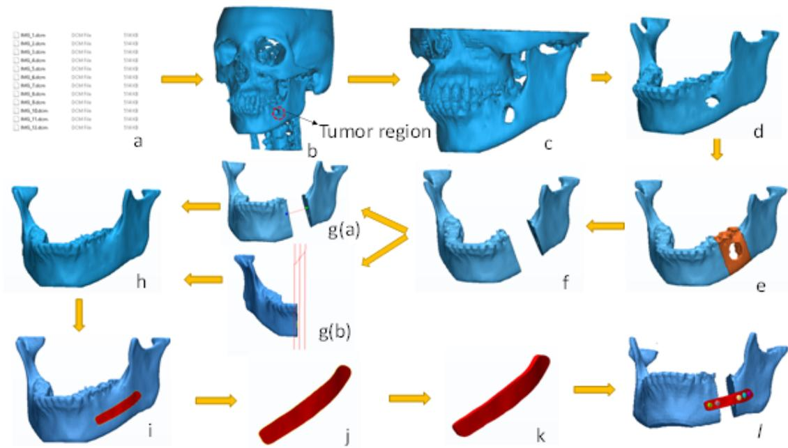
**Fig: 2.** Steps for the customized reconstruction plate design from DICOM files
