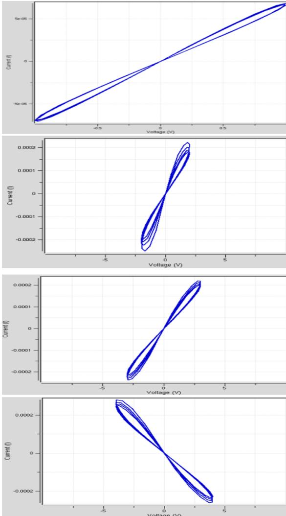
Fig8 VI curve at Input voltage 1v,2v,3v,4v at frequency 1Hz
