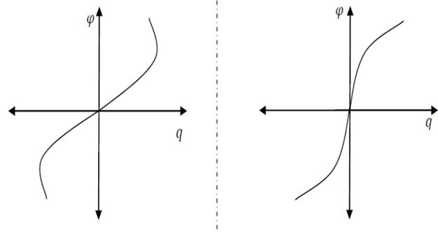
Fig5. Charge-flux characteristics of memristor[1]
