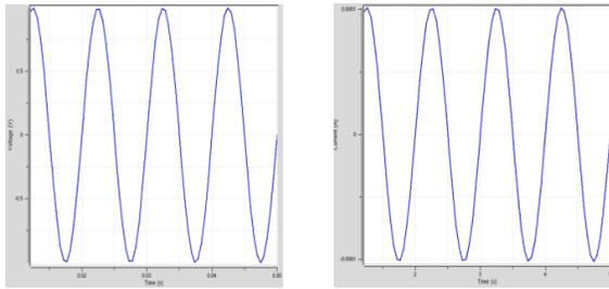
Fig3. Input voltage and output Current memristor
