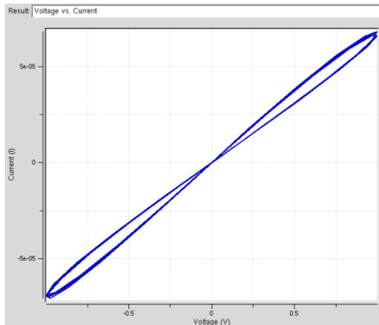
Fig5. Current –voltage characteristics of memristor
