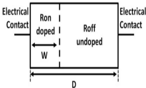
Fig4. Structure of memristor[2]
