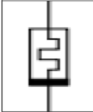
Fig.2 Symbol of memristor[1]
