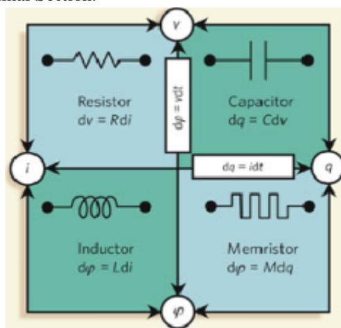
Fig1. Relation between four circuit variables
