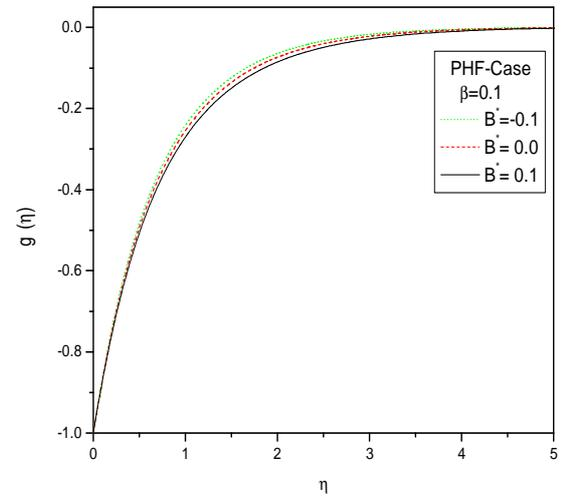
**Fig 13.** The effect of heat absorption  $B^*$  on the temperature profile for the PHF case at  $\beta = 0.1, Pr = 1, Ec = 0.2, A^* = 0.1$
