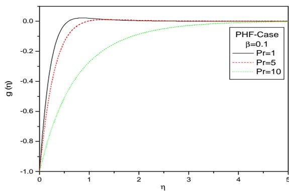
**Fig 7** The effect of Prandtl number  $Pr$  on the temperature profile for the PHF case at  $\beta = 0.1, Ec = 0.2, A^* = B^* = 0.1$
