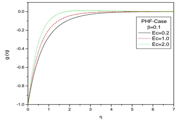
**Fig 9.** The effect of Eckert number  $Ec$  on the temperature profile for the PHF case at  $\beta = 0.1, Pr = 1, A^* = B^* = 0.1$
