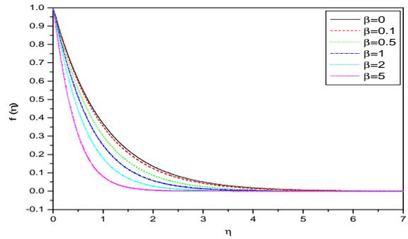
Fig 2 The effect of elastic parameter  $\beta$  on u-velocity component  $f$
