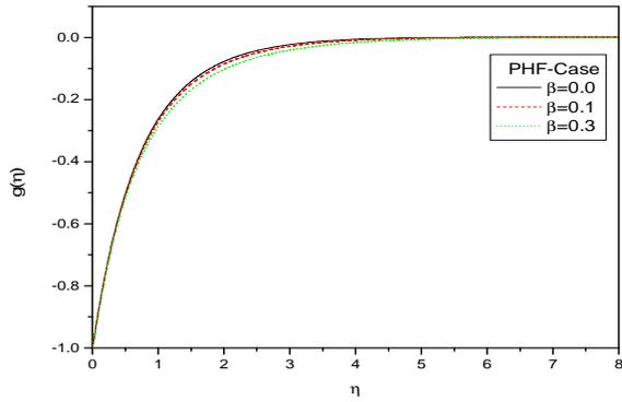
**Fig 5** The effect of elastic parameter  $\beta$  on temperature profile for the PHF case at  $Pr = 1.0, Ec = 0.2, A^* = B^* = 0.1$
