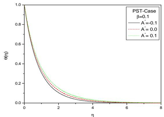
**Fig 10** The effect of heat generation  $A^*$  on the temperature profile for the PST case at  $\beta = 0.1, Pr = 1, Ec = 0.2, B^* = 0.1$
