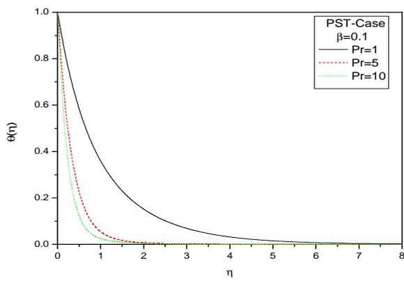
**Fig 6** The effect of Prandtl number  $Pr$  on the temperature profile for the PST case at  $\beta = 0.1, Ec = 0.2, A^* = B^* = 0.1$
