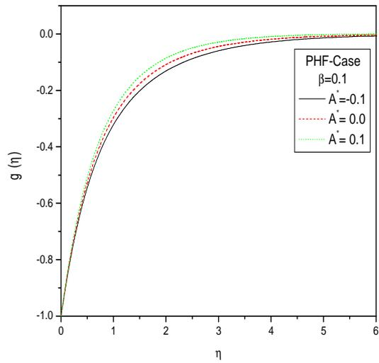
**Fig 11.** The effect of heat generation  $A^*$  on the temperature profile for the PHF case at  $\beta = 0.1, Pr = 1, Ec = 0.2, B^* = 0.1$
