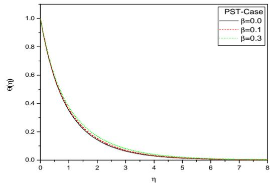
Fig 4 The effect of elastic parameter  $\beta$  on temperature profile for the PST case at  $Pr = 1.0, Ec = 0.2, A^* = B^* = 0.1$
