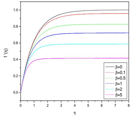
Fig 3 The effect of elastic parameter  $\beta$  on v-velocity component  $f'$
