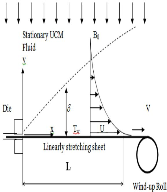
Fig.1. Schematic showing flow above a stretching sheet
