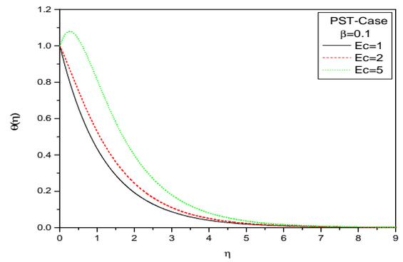
**Fig 8** The effect of Eckert number  $Ec$  on the temperature profile for the PST case at  $\beta = 0.1, Pr = 1, A^* = B^* = 0.1$
