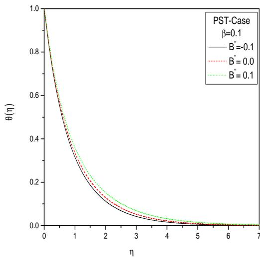
**Fig.12** The effect of heat absorption  $B^*$  on the temperature profile for the PST case at  $\beta = 0.1, Pr = 1, Ec = 0.2, A^* = 0.1$
