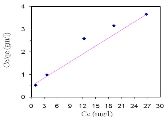
Fig.5: Langmuir isotherm for adsorption of MB on WHRP.
