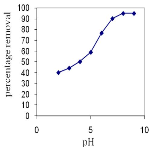
Fig.2: Effect of pH on percentage removal of MB (20mg/l) at room temperature.
