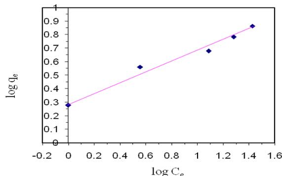
Fig.6: Freundlich isotherm for adsorption of MB on WHRP at room temperature.
