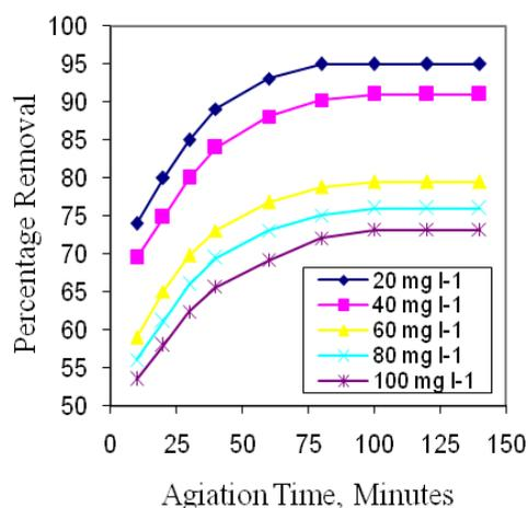
Fig.4: Effect of Initial Concentration and Contact Time on percentage removal of MB onto WHRP
