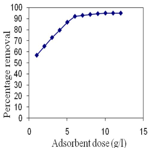
Fig.3: Effect of adsorbent dose on removal of MB for concentration 20mg/land 80 minutes agitation time at pH 8
