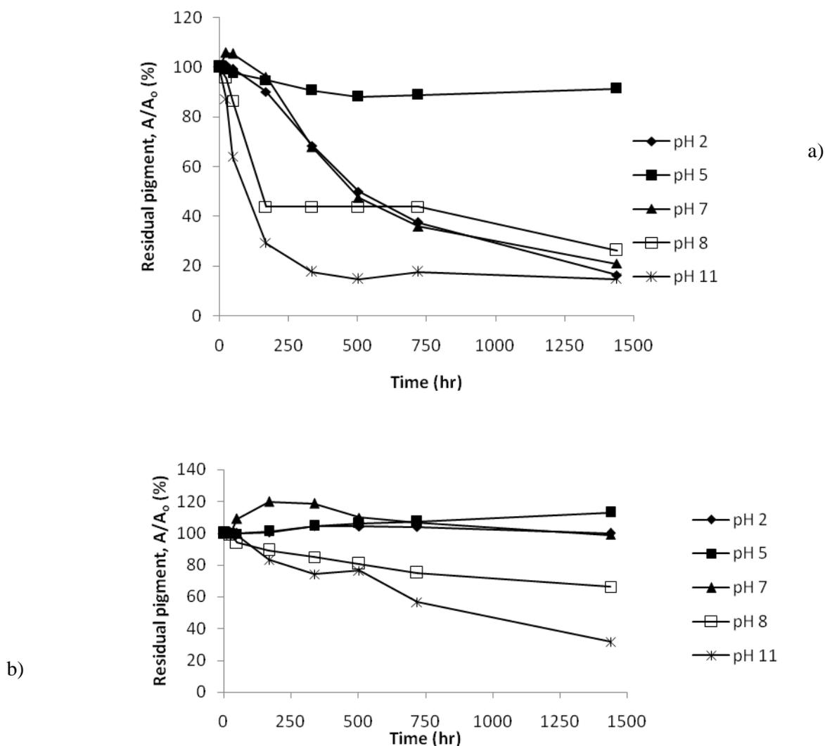
Figure 1: Stability of crude pigment at various pH upon exposure to fluorescent light (a) and kept in the dark (b) for 30 days
