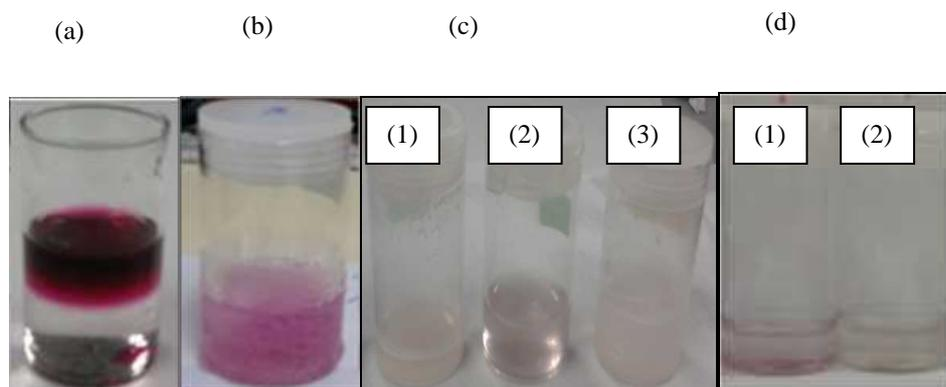
**Figure 6:** Effect of different solvents on crude and encapsulated prodigiosin (a) crude pigment in water, (b) encapsulated prodigiosin in water, (c) encapsulated prodigiosin in (1) acetone (2) n- hexane (3) ethyl acetate ,(d) encapsulated prodigiosin in (1) HCl (2) NaOH
