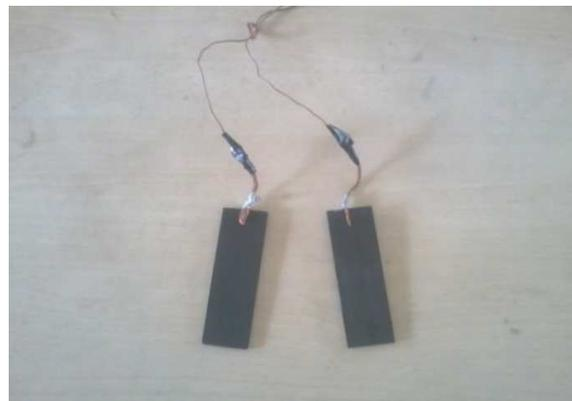
Fig.1: Graphite electrodes connected with wire.
