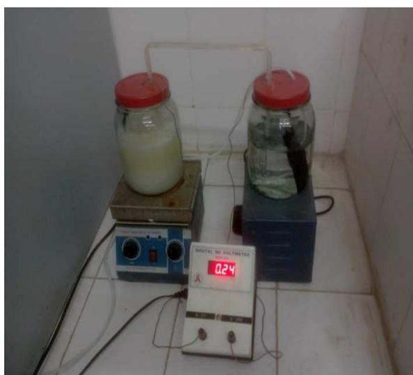
Fig.3: Experimental setup of MFC
