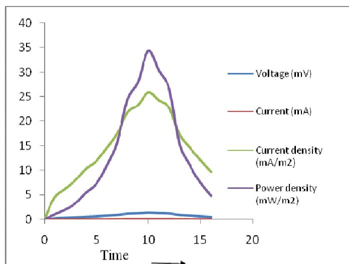
Graph 1 Results of MFC by using KOH electrolyte & Methylene Blue as mediator also use filming electrode
