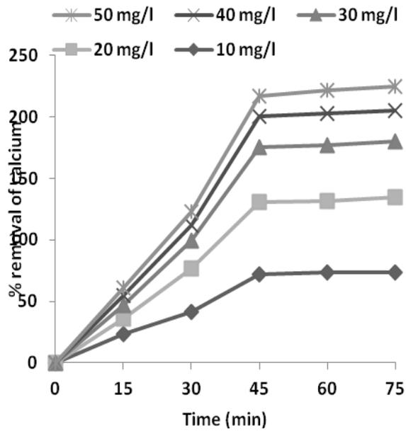
Fig. 2. Effect of contact time on removal of calcium in aqueous solution
