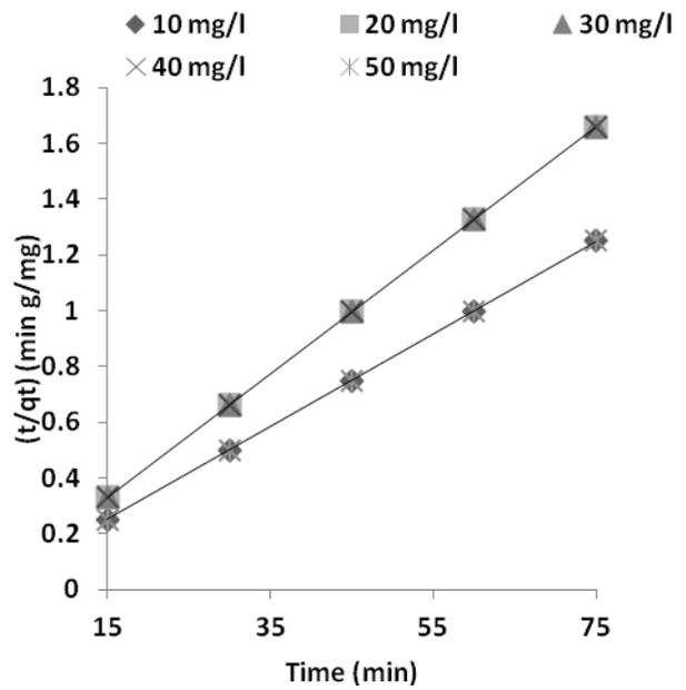
Fig.4. Kinetics analysis of calcium adsorption by linear plots of (pseudo second-order rate equations
