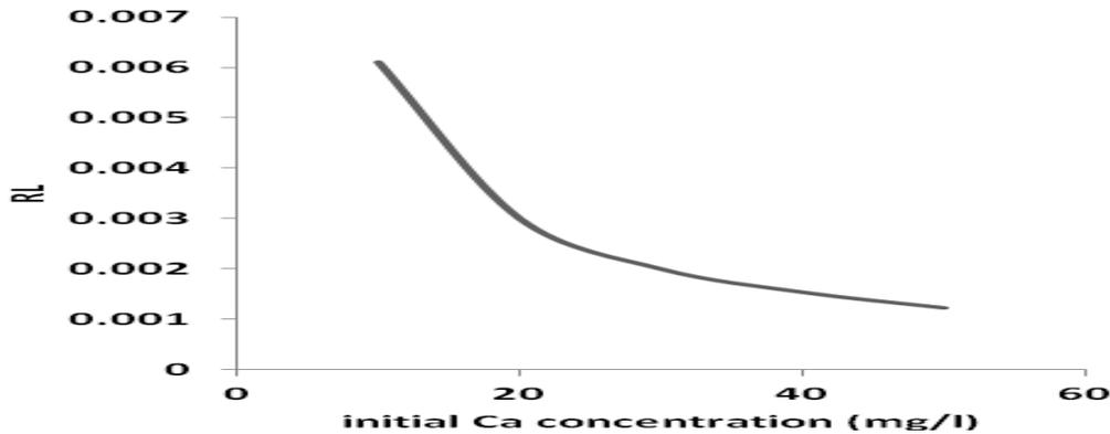
Fig. 12. Separation factor for calcium adsorption using *Gloeocapsa* sp.
