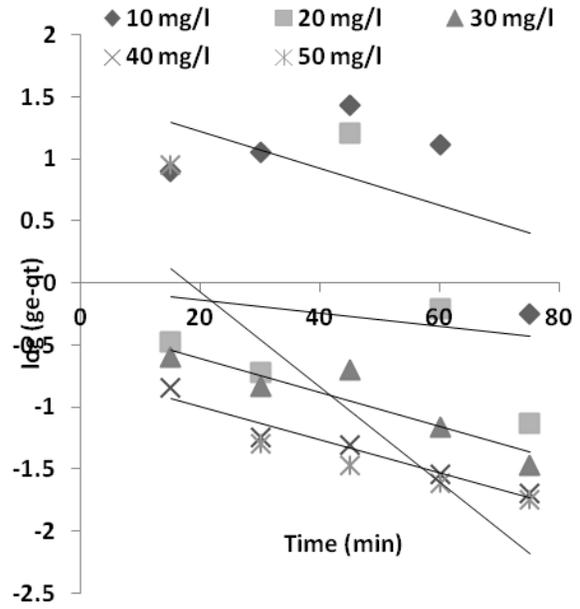
Fig.3 . Kinetics analysis of calcium adsorption by linear plots of (a) pseudo first-order rate equations
