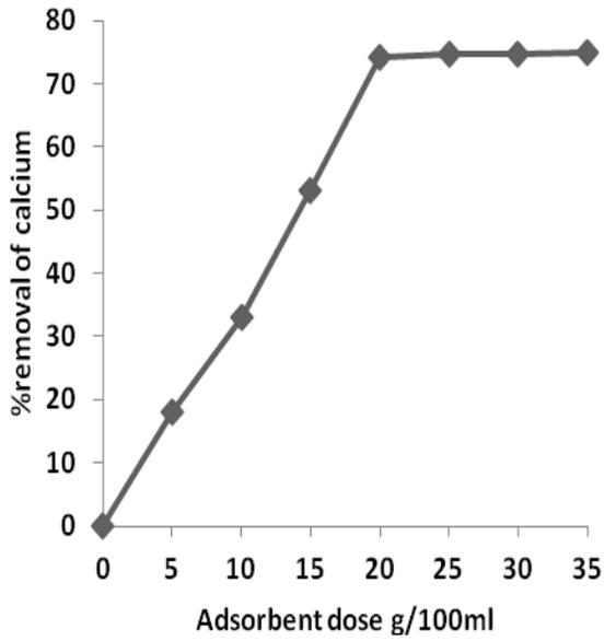
Fig 1. Effect of adsorbent dose on removal of calcium from sea brine solution
