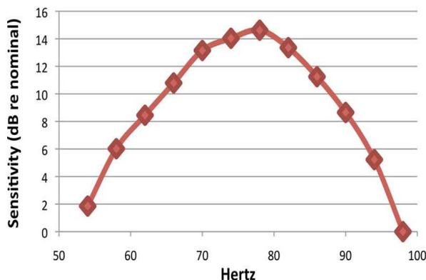
**FIGURE 4:-** Response curve between sensitivity and frequency for the sensing element that resonates at 78 Hz.
