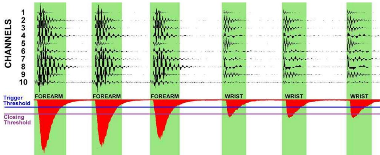
**FIGURE 7:-** Ten channels of acoustic data generated by three finger taps on the forearm, followed by three taps on the wrist.
