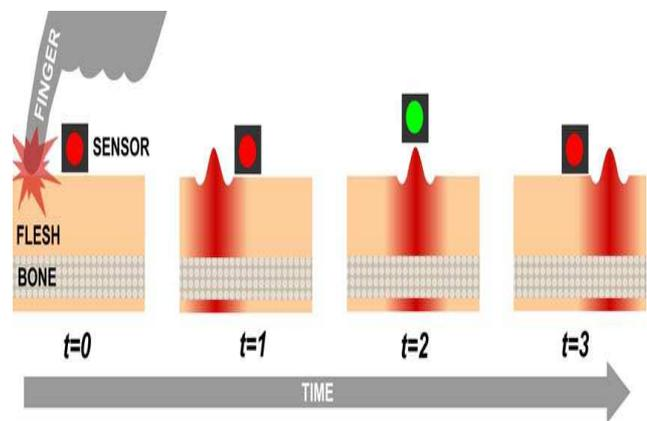
**FIGURE:-3(A):-** Transverse wave propogation:Finger impact displaces the skin,creating the transverse waves.
