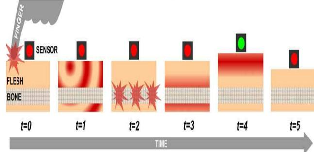
**FIGURE 3(B):-** Longitudinal wave propogation:Finger impact creates longitudinal waves that cause internal skeleton structures to vibrate.
