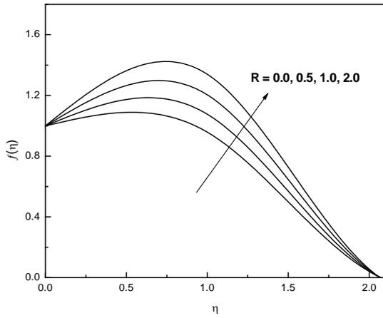
**Fig. 7:** Velocity Profiles for Different Values of  $R$
