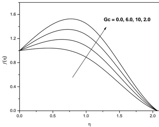
**Fig. 2:** Velocity Profiles for Different Values of  $Gc$
