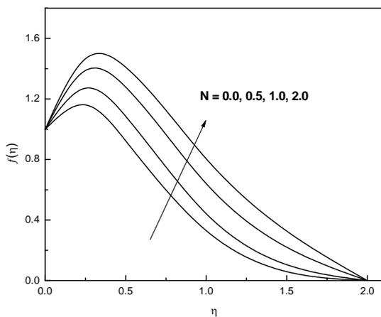
**Fig. 9:** Velocity Profiles for Different Values of  $N$
