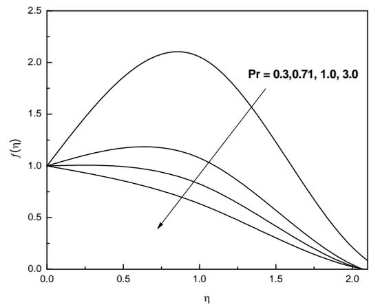
**Fig. 5:** Velocity Profiles for Different Values of  $Pr$
