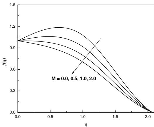
**Fig. 3:** Velocity Profiles for Different Values of  $M$
