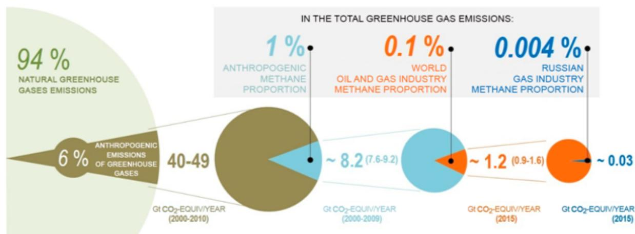
**Fig. 7.** The share of methane emissions from the gas industry in total greenhouse gas emissions
