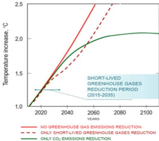
**Fig. 3.** Contribution of CO<sub>2</sub> and short-lived greenhouse gases to global temperature retention
