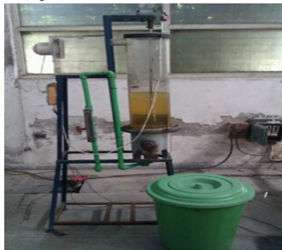
Main operation parameters that effect the frothier cell are Feed rate, Mineralogy, Particle size, pulp density and temperature.
