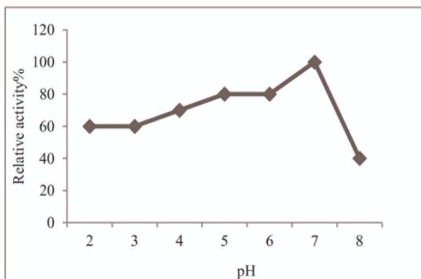
Fig. 4 Effect of pH on the biosensor
